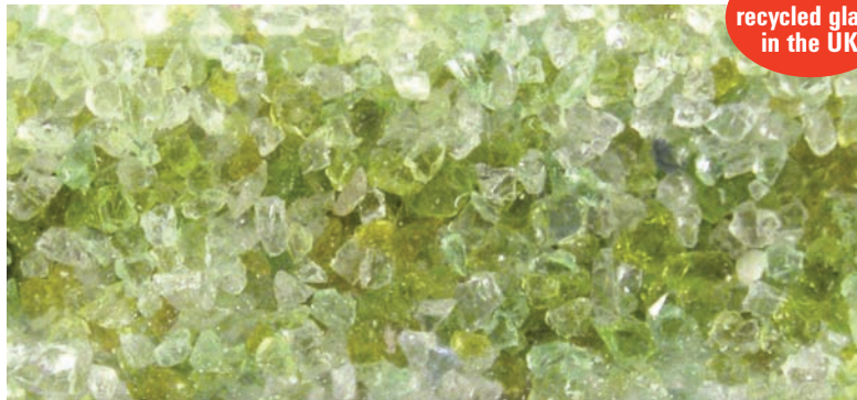
Grade 1 - equivalent to 16/30 grade sand
