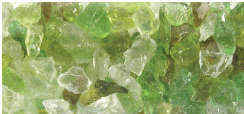
Grade 2 - equivalent to 8/16 grade sand
